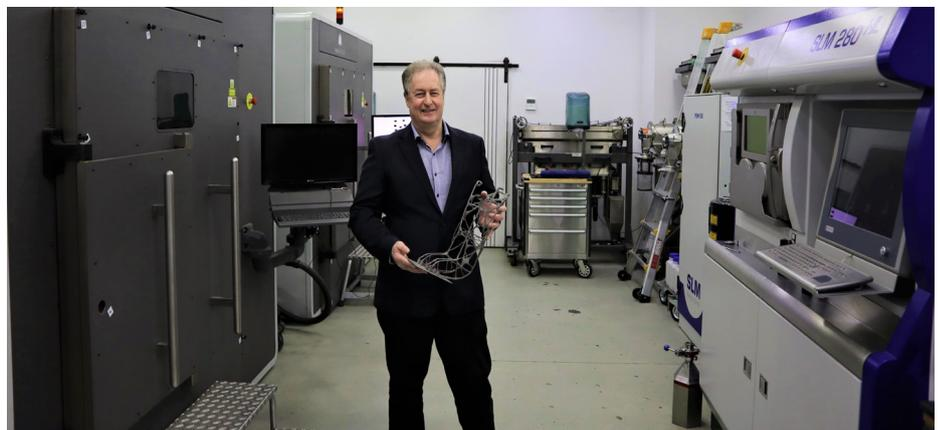
*Photo 1: Michael Bouchier showing a 3D printed pannier bracket for a high tech drone. We were able to reduce the weight from 4kg to 800g while increasing its strength compared to conventional products.*
