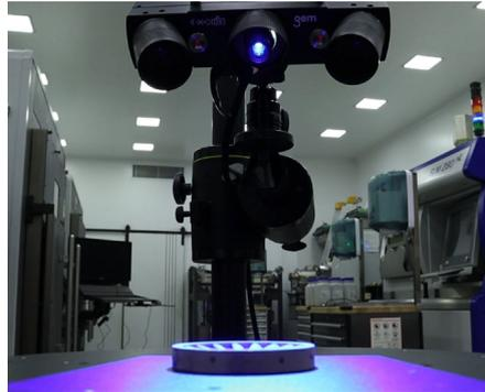
Photo 2: ATOS Q scanning metal printed turbine.
